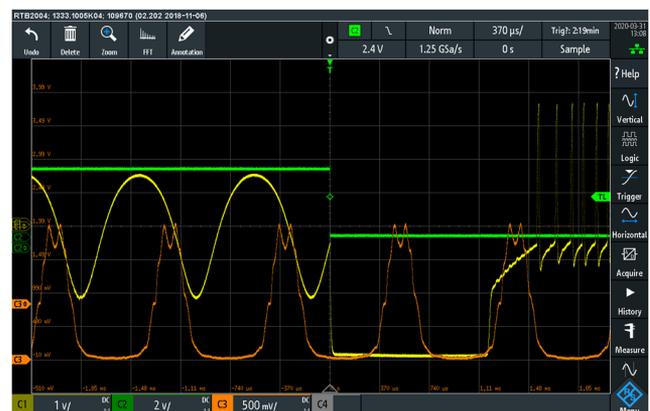
**FIG. 5.** Instantaneous shutdown of the autogeneration current through the wire. The time scale is  $370 \mu\text{s}$  per division. Electrical signal at the output of the autogenerator circuit amplifier (yellow; see item 8 in Fig. 4), the trigger signal to switch off the current through the wire (green), and the signal from the photodiode (orange). Measurements were made with the multichannel oscilloscope RTB2004.
