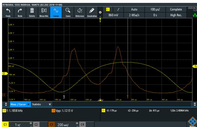
**FIG. 8.** One measuring period for the 7.15 mm position with a high resolution option of RTB2004: signal from the wire (yellow) and signal from the photodiode (orange). The measurements were made in the averaging mode with 2.5 (GSa/s), which in the high resolution option were averaged by the time period of 500 ns (corresponding to 2MSa/s).
