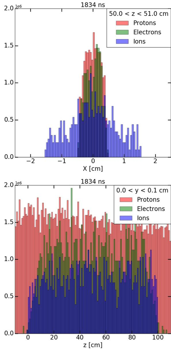
Figure 3: Distribution along  $x$  for the beam (red), electrons (green), and ions (blue) at the center of the Electron Column in  $z$  just before the beam would reenter the Column for a second pass - top. Note the beam distribution plotted is for the last time step that the beam is in the Column, for reference. Bottom - same as the top, but plotted along  $z$  at the center of the Column in  $y$ . The bin widths correspond to the simulation grid spacing.
