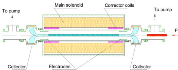
Figure 1: Schematic of the Electron Column in IOTA.
