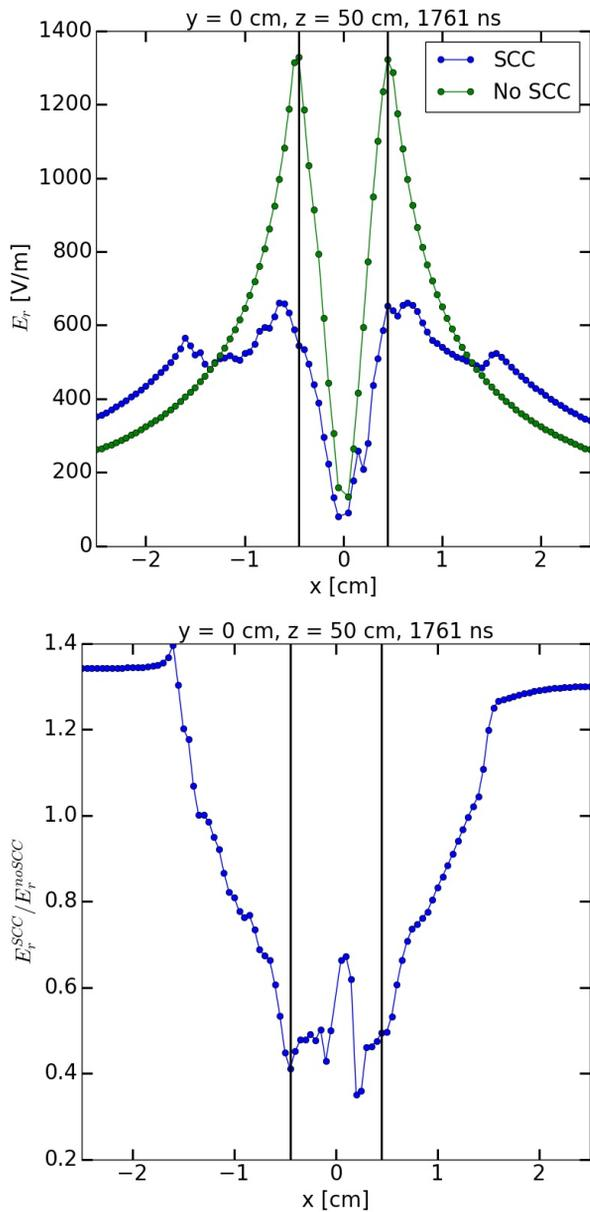
Figure 2: Radial electric field along  $x$  in the center of the column in  $y$  and  $z$  for beam alone (green) and with space-charge compensation (blue) at the end of the first pass of the beam through the Electron Column - top. Ratio of the two electric fields from the top plot - bottom. The vertical lines in both plots denote the boundary of the beam.
