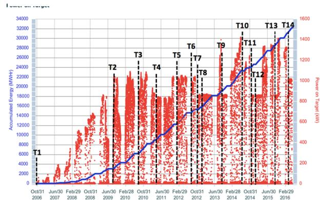
5000 MW-hr design, two recent target failures – costly to replace (1 M\$, 1 week)
