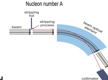
for partially stripped ion beams: The collimation of partially stripped ions relies on the change of the charge state using a stripping foil →
