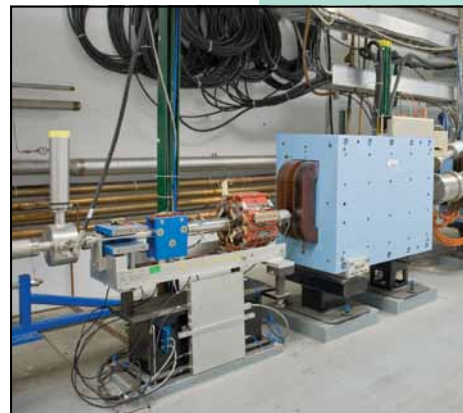
B, C. Magnets and vacuum chambers at Jefferson Laboratory. Visible here are a focusing magnet (red), a bending magnet (light blue) and the stainless steel vacuum chamber (beam pipe).
