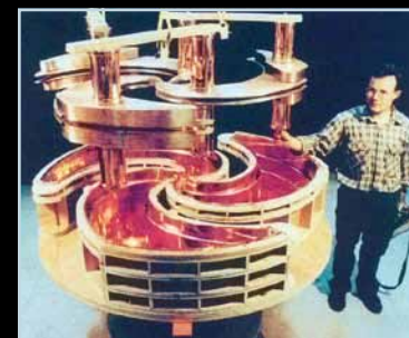
Full-scale model of the radio-frequency cavity of a superconducting cyclotron design of the AIMA Company for high-energy proton therapy.
