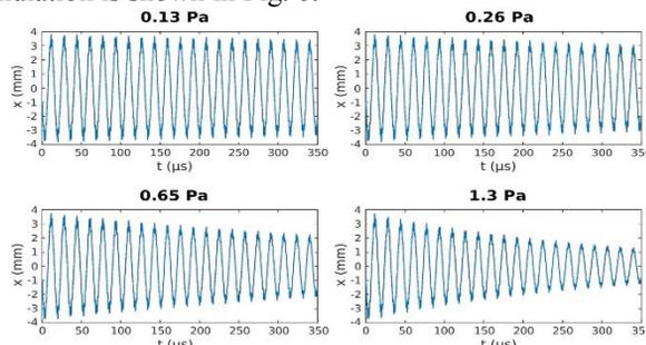
Figure 6: The motion of an ion simulated by G4beamline, varying the pressure of the buffer gas.
