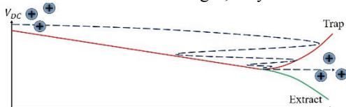
Figure 3: Potential well by the segmented electrodes and movement of ion along axial direction.
