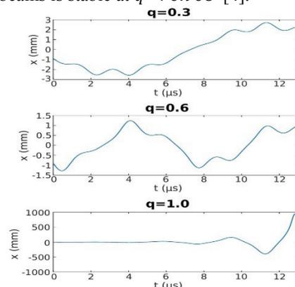
Figure 1: Graphs of the motion of an ion in the RFQ with various  $q$  obtained by G4beamline.
