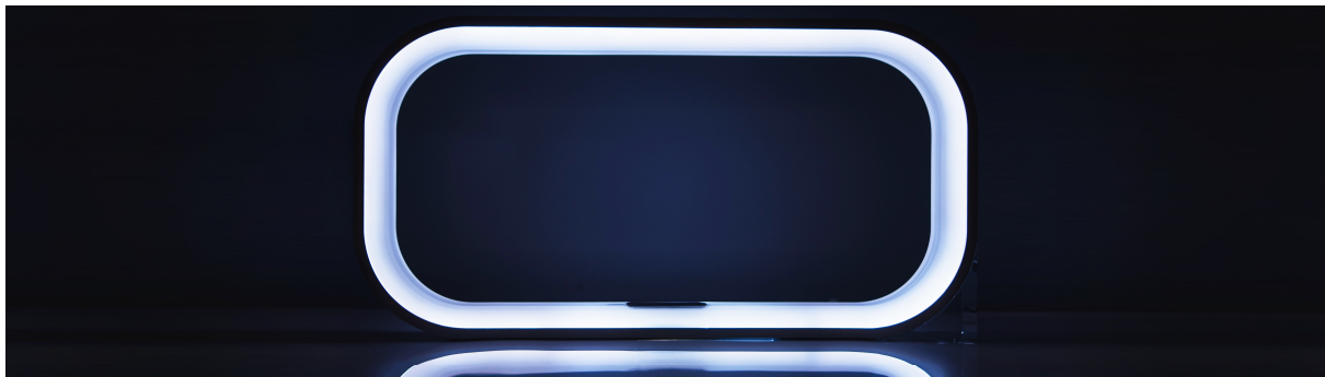
Figure 1. Hand-in-O prototype. The perforated space inside the frame is large enough to put both hands in. Light comes from inside the frame, and there is a Leap Motion at the bottom of the frame that can recognize hand gestures.
