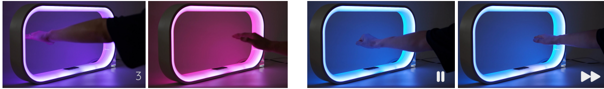
Figure 2. Gesture interaction and light feedback in the context of music control. Left - The color of light changes when users put their hand to each side in the frame for more than 3 seconds; Right - the song pauses when the user clenches a fist and fast-forwards when the user moves the hand to the right.
