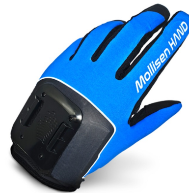
Soft sensor embedded glove <출처 : https://kr.ftsame.com >
