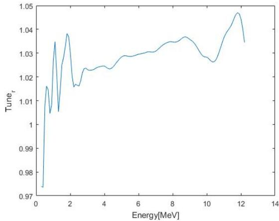
Figure 5: Radial tune variation with respect to beam energy.
