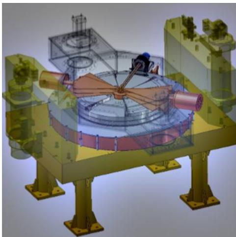
Figure 1: 13 MeV cyclotron.
