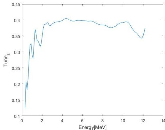
Figure 6: Vertical tune variation with respect to beam energy.
