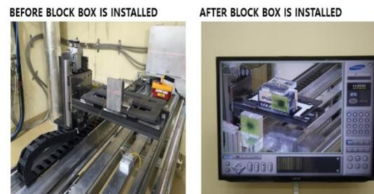
Figure 2: Before box is installed to block the convection vs after it is blocked.
