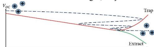
Figure 3: Potential well by the segmented electrodes and movement of ion along axial direction.
